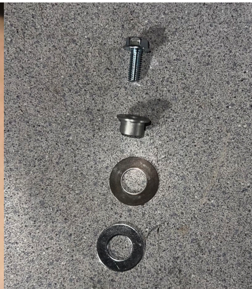
Fig. 5 (EFI Pump/Metal OEM Flange-Ring/IMS Flat Washer/OEM Crush Washer/OEM Sleeve Combo)
